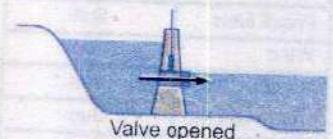
Low tide: Water is beginning to flow out of basin to ocean, driving turbines.
