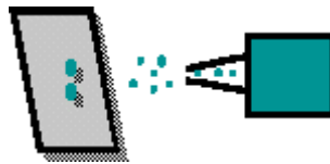
Figure 2.36 "Internal Functionality of an Ink-Jet Printer"
